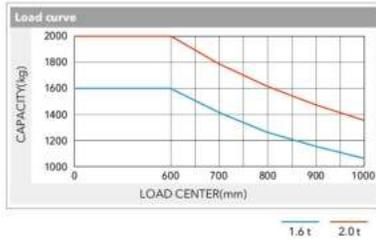
Note: The vertical axis stands for load capacity and the horizontal axis stands for load center which is calculated from the front surface of the forks to the gravity of the standard load. The standard load means a cubic with 1000mm edge length. When mast is tilted forward, using non-standard forks or loading large goods, the load capacity will be reduced. The load capacity of standard mast at different load center can be known from this load chart.
